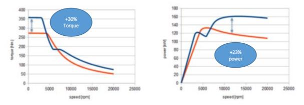
The Coil Driver takes each coil and breaks it into two or more coils. The switching circuitry puts the coils in series, parallel, or a combination, depending on load and speed demands at that moment. When the coils are in series, the Page 2
